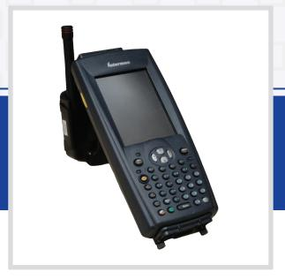
Built on Savi's active RFID technology, the Savi Handheld Reader Kit with Intermec Mobile Computer 7X1 Series is designed to help users quickly locate, identify and track supply chain assets in austere environments. The handheld kit can read from and write to active, data-rich RFID tags, and can also scan and process data from standard linear, matrix, 1D and 2D bar code. The handheld kit is packaged with options that provide specific components based on the needs of the customer.
