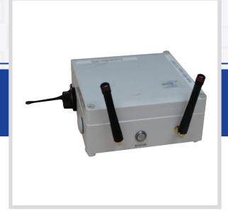
Unlike the Savi Signpost (SP-651), the Savi Signpost-Reader (SP-652) includes a built-in ISO 18000-7 reader. The Savi Signpost-Reader enhances ISO 18000-7 compliant installations by working together with Savi's RFID tags and readers. Signpost-Readers provide a low frequency (LF) wake-up capability that allows for the precise location and identification of assets as they pass through gates and chokepoints
