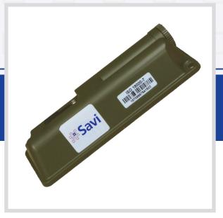
The Savi ST-618 is a rugged active RFID tag ideally suited for the locating, tracking and managing of medium to high value assets in both defense and commercial applications. The ST-618 carries enough memory to record asset configuration and maintenance records, and is ideal for these functions.
