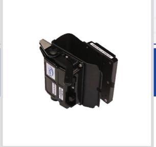
The Savi ST-675 is an active RFID container security tag with intrusion and environmental sensors. The ST-675's sensor arm detects the open/closed state of the shipping container door, and the intrusion light sensor monitors the amount of light entering the container. These intrusion sensors detect potential theft or tampering. The temperature, humidity and shock sensors monitor environmental conditions to prevent spoilage and damage to goods.
